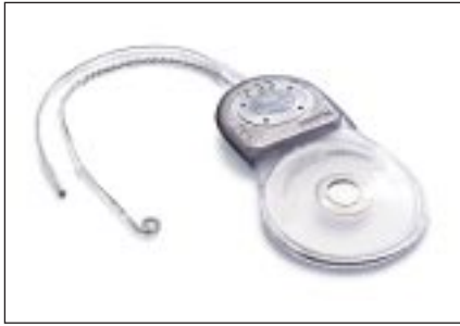
Figure 4: The internal portion of the cochlear implant is seated within the thickness of the cranial vault and has both a cochlear and a ball electrode.
