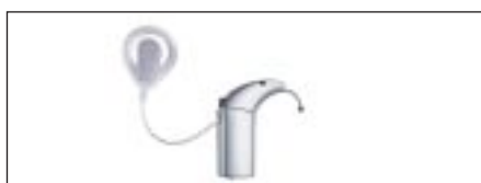
Figure 3: External component of the cochlear implant - Newer smaller ear-level device.
