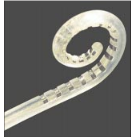
Figure 6: The most advanced cochlear implant has a pre-curved electrode permitting it to lie closer to the cochlear nerve.
