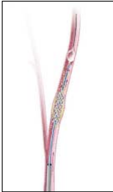
Figure 2a: Demonstrates the action of the Distal Balloon in Preventing Embolization During a Stent Procedure
