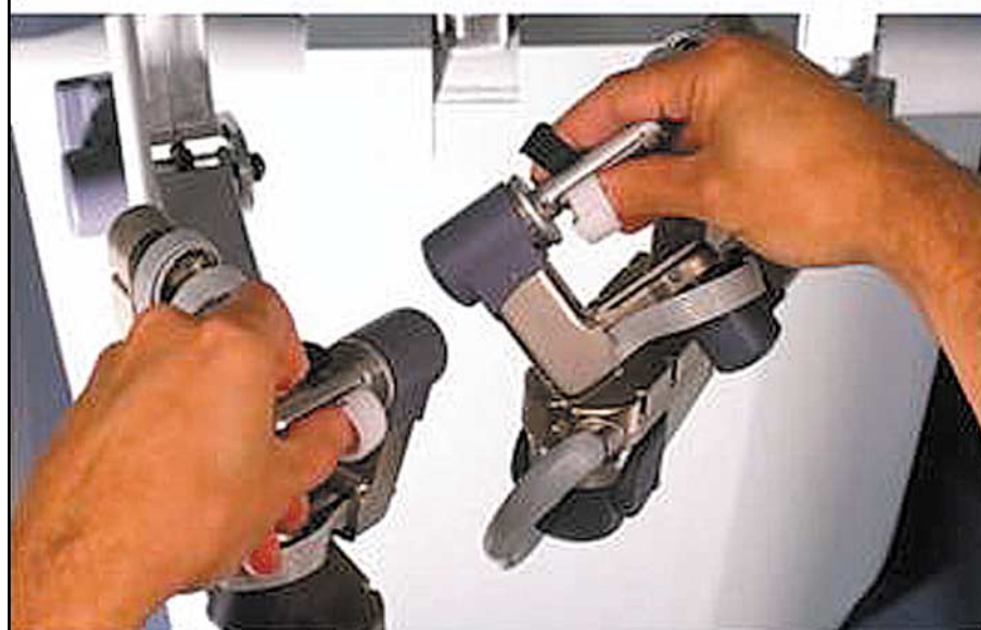
Figure 1b: Surgeon's wrist and finger movements are translated to the articulated instruments attached to robotic arms within the patient.
