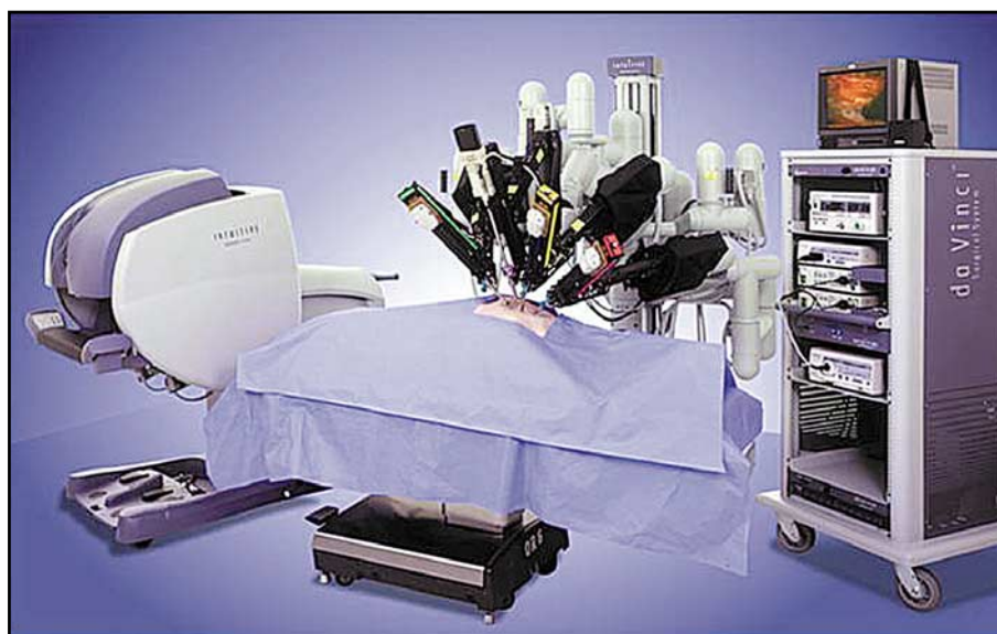
Figure 1a: Surgeon's Console (left), da Vinci Robot arms in patient (centre) and Vision Cart (right)
